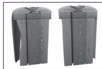
Figure 2. Improvements in nasal actuator moulding quality a result of optimisation following x-ray analysis (left → right).
